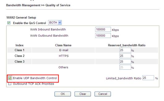
9. If the worker has connected to the headquarter using host to host VPN tunnel. (Please refer to Chapter 3 VPN for detail instruction), he may set up an index for it. Enter the Class Name of Index 3. In this index, he will set reserved bandwidth for 1 VPN tunnel.
