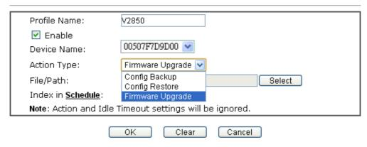
In the field of Profile Name, type a name for such maintenance profile; check Enable; and choose the one you want to perform firmware upgrade from Device Name drop down list. From the Action Type, choose Firmware Upgrade. Type the file/path of the newest firmware or click Select to locate it. Specify the Schedule profile. At last, click **OK**.
