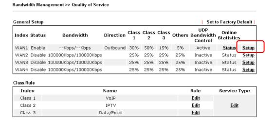
10. In the Setup page, check the box of **Enable the QoS Control**. Type 30, 50 and 15 in the boxes for VoIP, IPTV and Data/Email respectively. Check the box of **Enable UDP Bandwidth Control**.
