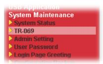
3. In the field of ACS Server, type the URL (IP address with port number) of Vigor2860 series and type the same Username and Password defined on the page of Central VPN Management>>General Setup in Vigor2860 series. Then, click Enable for CPE Client and then click OK to save the settings.
