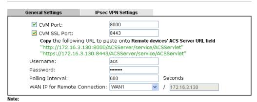
To enable the CVM feature, one of the Port MUST be Enabled!
