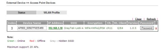
In this case, a device named with AP800\_00507F6EE4980 has been detected by Vigor router.
