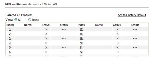
3. Click any index number to open the configuration page. Type a name which is easy for identification for such profile (in this case, type *VPN Client*), and check the box of **Enable This Profile**. For such Vigor router will be set as a **client**, the call direction shall be set as **Dial-out**. Check the box of **Always on** for a permanent VPN connection.
