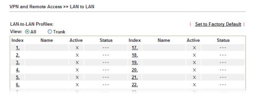
3. Click any index number to open the configuration page. Type a name which is easy for identification for such profile (in this case, type *VPN Server*), and check the box of **Enable This Profile**. For Vigor router will be set as a **server**, the call direction shall be set as **Dial-in** and set 0 as **Idle Timeout**.
