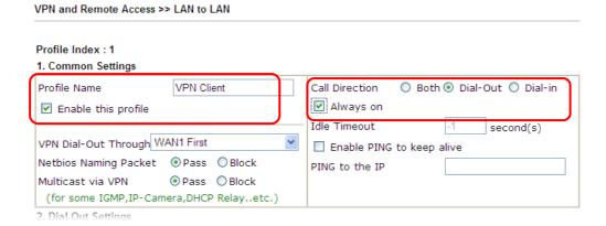
4. Now navigate to the next section, **Dial-Out Settings** to select the **IPsec Tunnel** service and type the remote server IP/host name (e.g., 218.242.133.91, in this case). Press the **IKE Pre-Shared Key** button to set the **PSK**; and select **Medium (AH)** or **High (ESP)** as the security method.
