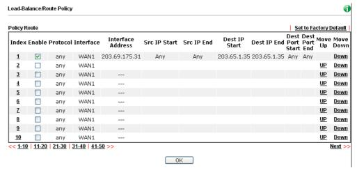
Now, the packets sent to the remote PC (IP address: 203.65.1.35) will be forcefully to pass through WAN1.
