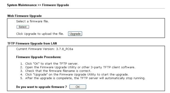
Choose the right firmware by clicking **Select**. Then, click **Upgrade**. The system will upgrade the firmware of the router automatically.
