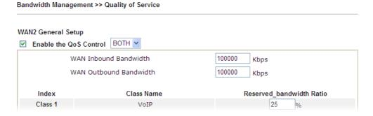
**Note:** The rate of outbound/inbound must be smaller than the real bandwidth to ensure correct calculation of QoS. It is suggested to set the bandwidth value for inbound/outbound as 80% - 85% of physical network speed provided by ISP to maximize the QoS performance.
