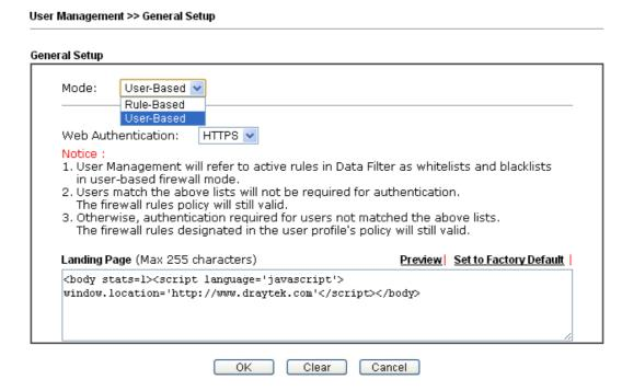
With **User Management** authentication function, before a valid username and password have been correctly supplied, a particular client will not be allowed to access Internet through the router. There are three ways for authentication: **Web**, **Telnet** and **Alert Tool**.
