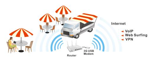
After connecting into the router, 3G/4G USB Modem will be regarded as the WAN3/WAN4 port. However, the original WAN1 and WAN2 still can be used and Load-Balance can be done in the router. Besides, 3G/4G USB Modem in WAN3/WAN4 also can be used as backup device. Therefore, when WAN1 and WAN2 are not available, the router will use 3.5G for supporting automatically. The supported 3G/4G USB Modem will be listed on DrayTek web site. Please visit www.draytek.com for more detailed information.
