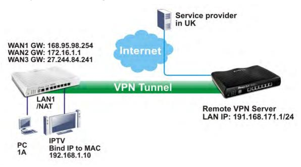
A VPN tunnel has been established between Router A and router B.
