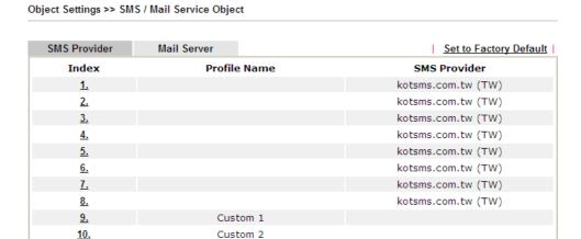
Index 1 to Index 8 allows you to choose the built-in SMS service provider. If the SMS service provider is not on the list, you can configure Index 9 and Index 10 to add the new service provider to Vigor router.
