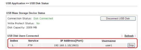
Now, users in LAN of Vigor2710 can access into the USB storage device by typing ftp://192.168.1.1 on any browser. They can add or remove files / directories, depending on the Access Rule for FTP account settings in USB Application >> USB User Management.
