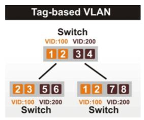
Vigor routers [Note] support Tag-based feature both on LAN and WAN interfaces. The next we'll demonstrate our web design and how to configure the settings by introducing the functionalities of Vigor router.
