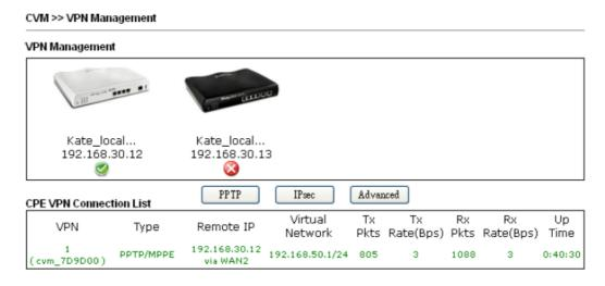
5. A LAN to LAN profile for such VPN will be generated automatically. You can access into **VPN and Remote Access>>LAN to LAN** of the remote device for viewing the detailed information.
