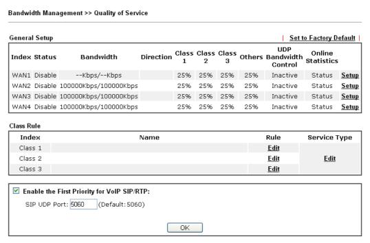
2. Click **Setup** link of WAN(1/2/3). Make sure the QoS Control on the left corner is checked. And select **BOTH** in **Direction**.
