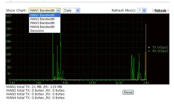
The horizontal axis represents time. Yet the vertical axis has different meanings. For WAN1/WAN2/WAN3/WAN4 Bandwidth chart, the numbers displayed on vertical axis represent the numbers of the transmitted and received packets in the past.
